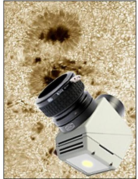
The Baader Safety Herschel-Prism features a ceramic window which works as Solar finder screen and “heat cage” at the same time. Due to the closed design of the magnesium prism body there is no dangerous amount of light exiting the Baader Safety Herschel-Prism. Due to this improvement the Herschel-Prism evolves into a safe device for Solar observation – even and especially for educational purposes.
