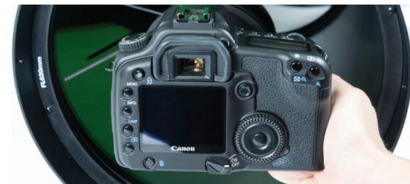
4. Finish threading the retaining ring onto the telescope. Turn until the camera adapter is snug against the telescope. Do not over tighten! Camera orientation can be adjusted later.
