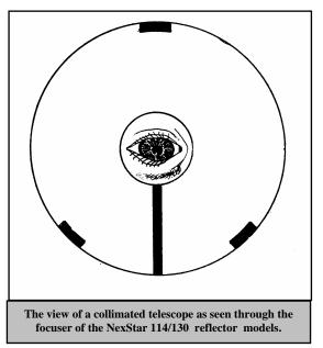
If your telescope is out of collimation, the best way to re-collimate it is
