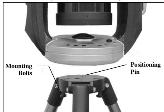
**Figure 3-2 Mounting the Telescope**
