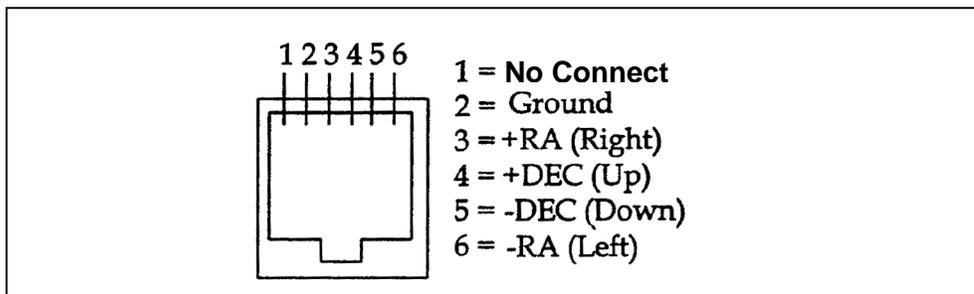
**Figure 8-7 – Pin out diagram for Autoguider**
