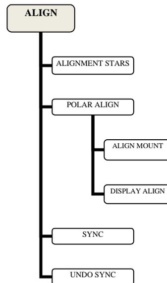
2. Slew the telescope to one of the original alignment stars, or another bright star if the original alignment stars are no longer in a convenient location. Press the *Align* button and use the Up/Down buttons on the hand controller to select *Alignment Stars* from the list.
