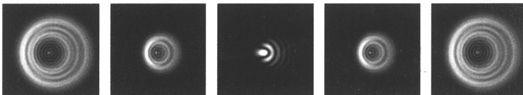
**Figure 9-2 -- Even though the star pattern appears the same on both sides of focus, they are asymmetric. The dark obstruction is skewed off to the left side of the diffraction pattern indicating poor collimation.**
