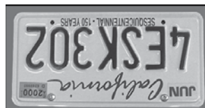
Inverted image, as viewed with the eyepiece directly in telescope
