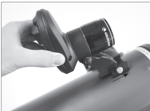
Installing small base (back to front)
