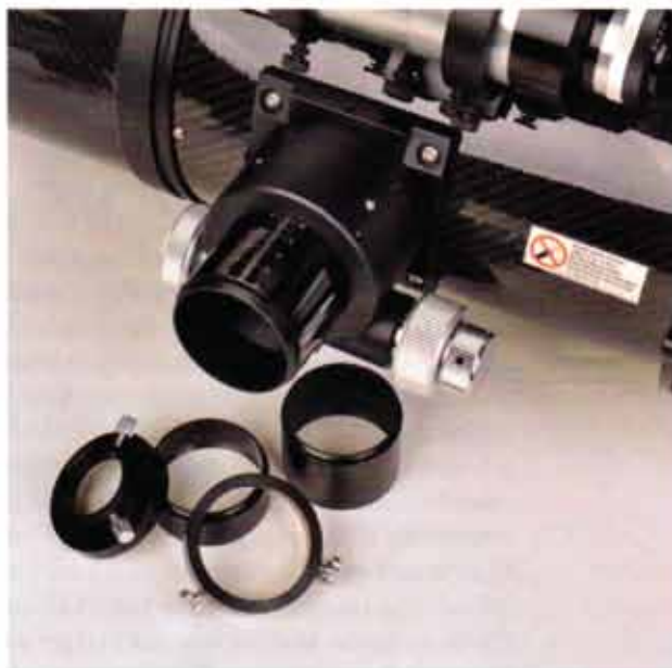
The dual-speed Crayford-style focuser comes with two extension tubes and adapters for 1 1/4- and 2-inch eyepieces. The scope's focal point falls approximately 3 1/4 inches (95 mm) beyond the top of the focuser's body.
