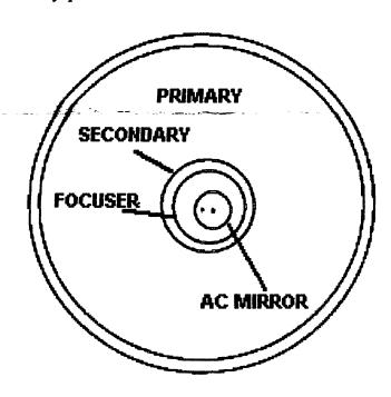
The drawing at the left represents the view when looking through the autocollimator. The outer circle is the aperture at the end of the scope. The dot in the center of the auto collimator mirror is the reflection of the perforation at the eye end. The spot to the left represents the dot on the center of the primary in a slightly out of collimation system.
