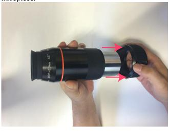
3. Slip the provided ring over the nosepiece and tighten as shown.
