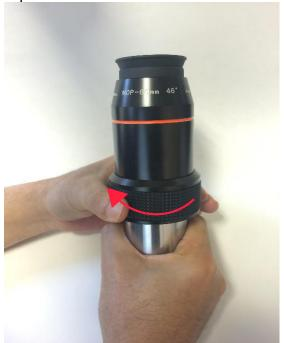
2. Hold the eyepiece by its body and remove the rubber grip by pulling it past the end of the nosepiece.
