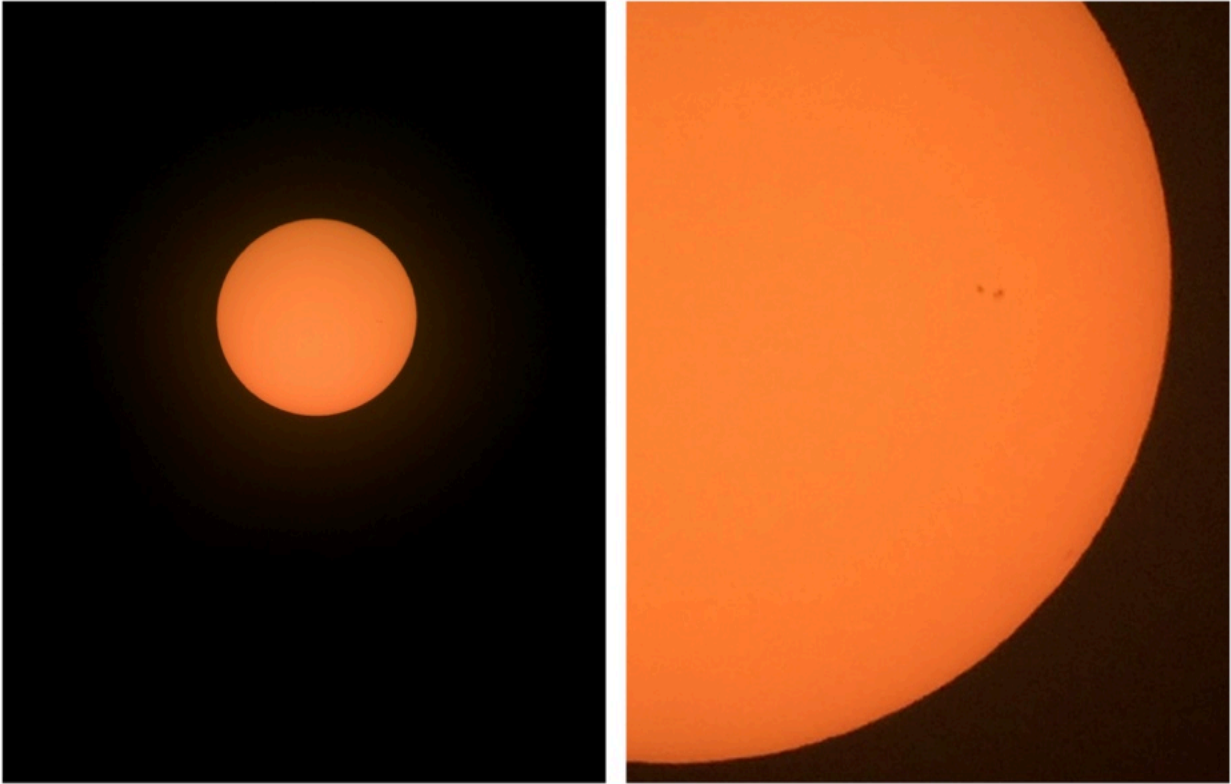
Figure 7-6: Uncropped afocal images of the Sun taken with a smartphone held with a holder/bracket at an eyepiece with focal length of 18.2mm and a telescope with 80mm objective lens and focal length of 480mm. A polymer solar filter was used over the objective lens of the telescope. The image on the left was taken with the smartphone camera set to lowest zoom setting. The image on the right was taken with the smartphone camera set to highest zoom setting. The camera automatically set the exposure. Credit: Sergio Castillo/Agenda Astro.
