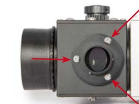
The screws for adjusting the bottom port of the BFM II.
