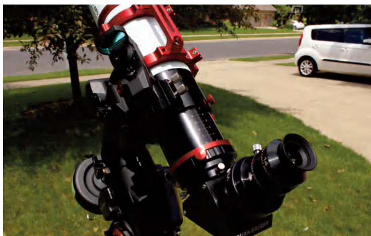
Image 5 - The telescope comes with a finder scope shoe. The red knob near the diagonal allows for 360 rotation of the diagonal.
