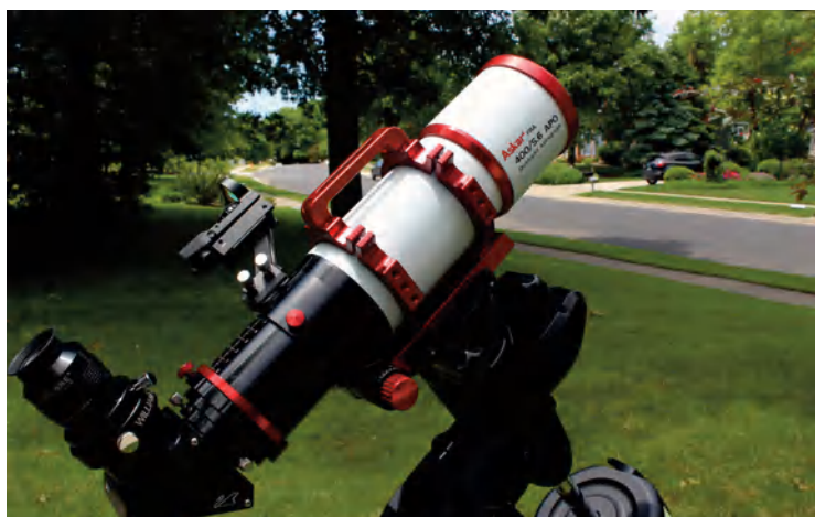
Image 4 - View with the focuser draw tube fully extended. The black knob is the course focus knob while the red one is for fine focus.
