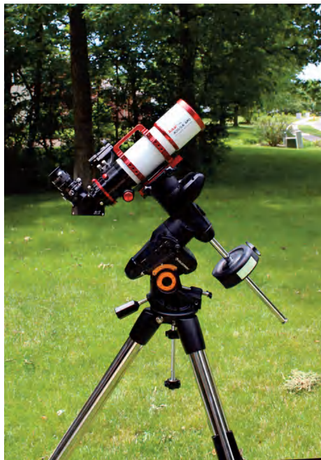
Image 1 – The Askar FRA 400 telescope atop a Celestron Advanced VX mount.
