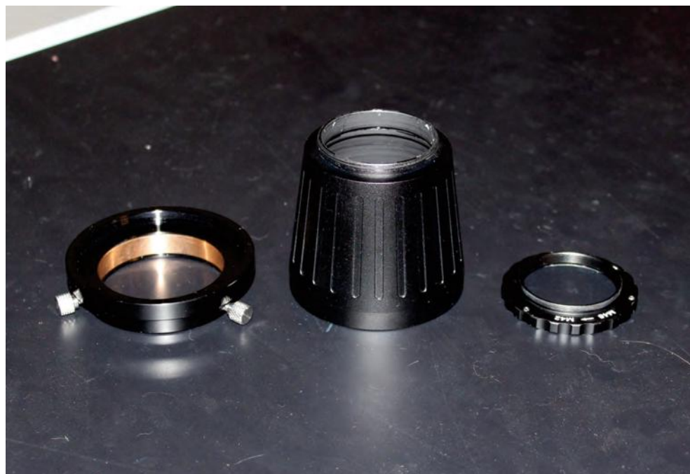
Image 14 - The accessory on the left screws onto the end of the focuser to attach a 2-inch diagonal or a 2-inch to 1.25-inch adapter to use with a 1.25-inch diagonal. The accessory in the middle screws onto the end of the diagonal to connect to a camera with M48 threads. The adapter on the right is the author's M48-M42 adapter allowing him to attach his CCD cameras to the telescope.
