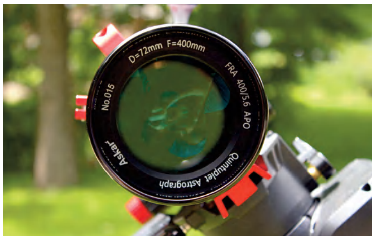
Image 3 - The quintuplet optics has five elements in two groups with two extra-low dispersion lenses.
