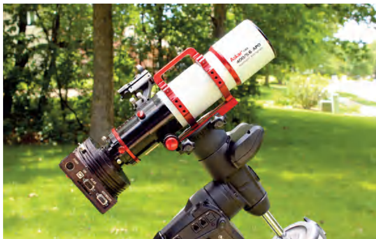
Image 7 - With the SBIG ST-2000XCM CCD camera, the telescope dovetail plate and tube rings must place the telescope as high up on the mount as possible to balance the declination axis.
