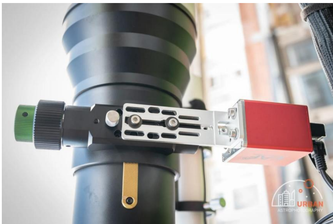
A ZWO EAF fits onto the focuser very easily.
