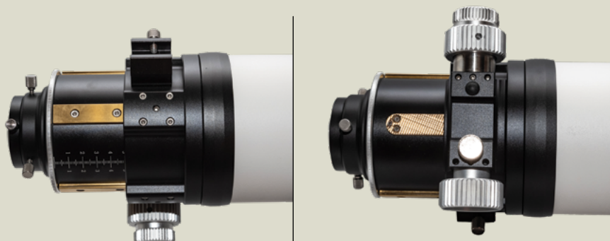
▲ Left: The rack-and-pinion focuser rides along three linear bearings that produce excellent rigidity. Right: a knurled thumbscrew located on the bottom of the gearbox locks the focuser in place.
