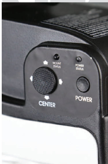
The eight-position joy stick provides pinpoint targeting of solar features
