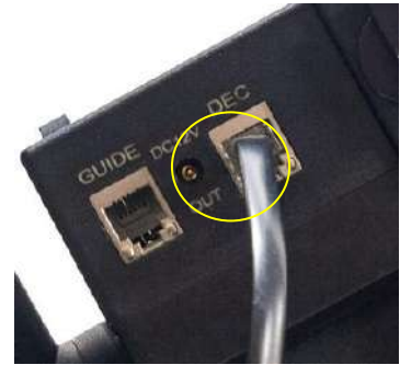
Figure 2. Connect polar scope LED
