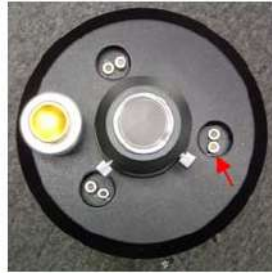
Figure 6b. Now, turn the push screw in the same set clockwise no more than \frac{1}{4} turn.
