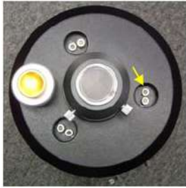
Figure 6a. Turn the pull screw counterclockwise a small amount, no more than a \frac{1}{4} turn. (Note: actual selected alignment screw will vary.)
