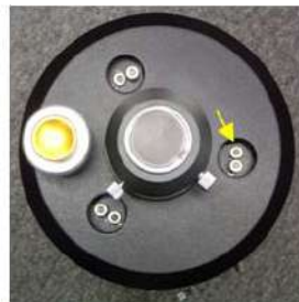
Figure 7b. Now, turn the pull screw in the same set clockwise no more than \frac{1}{4} turn.
