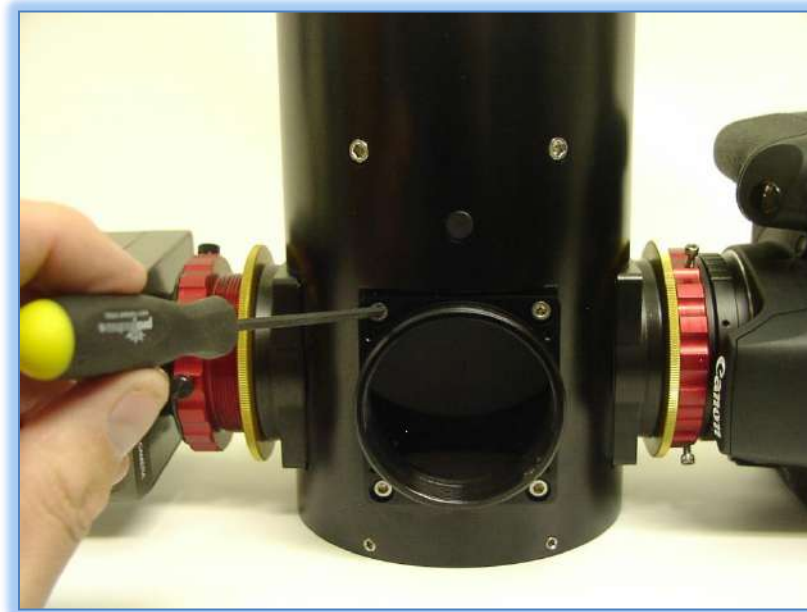
Adjusting the 2-inch saddle in X-Y directions.
