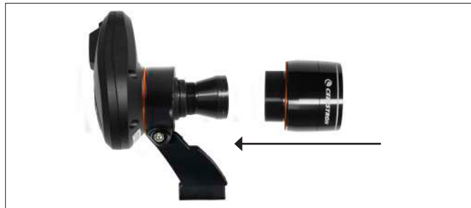
Fig. 9: Reinstall the front housing onto SSAA. Don't forget the orange cosmetic ring!
