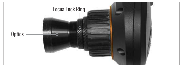
Fig. 24: Loosen the lock ring when making focus adjustments, then firmly retighten when focused.
