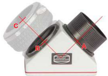
The required backfokus can be reduced from 112 mm with ClickLock® (A-C) to ca. 71,5 mm without ClickLock® (A-B).
